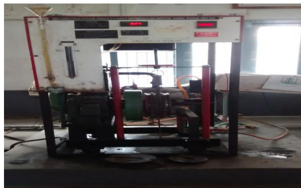
Fig:4 Experimental setup of four stroke, single cylinder, water cooled diesel engine.
